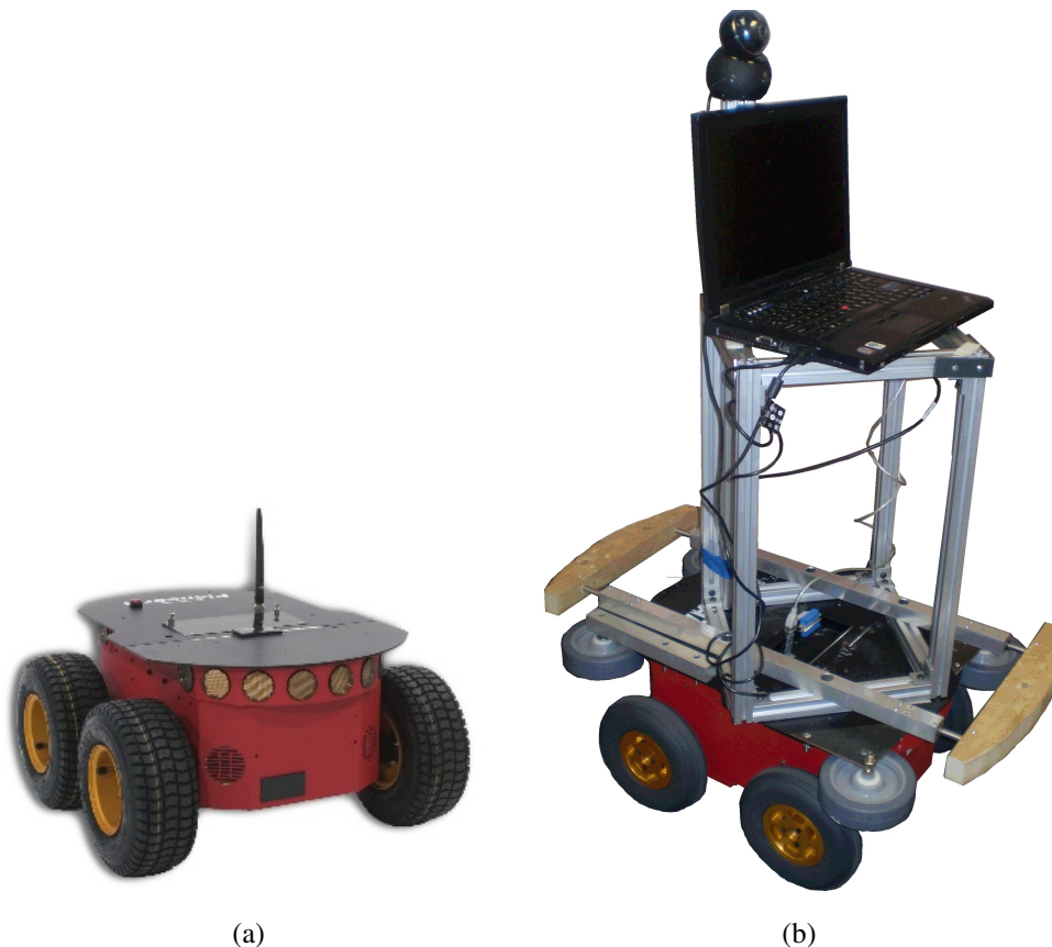
Figure 1.1: (a) The Pioneer 3-AT robot; (b) the extended Pioneer 3-AT robot.
