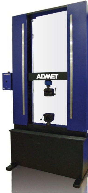
Figure 1.3: Picture of the eXpert 2653 ADMET universal testing machine.
